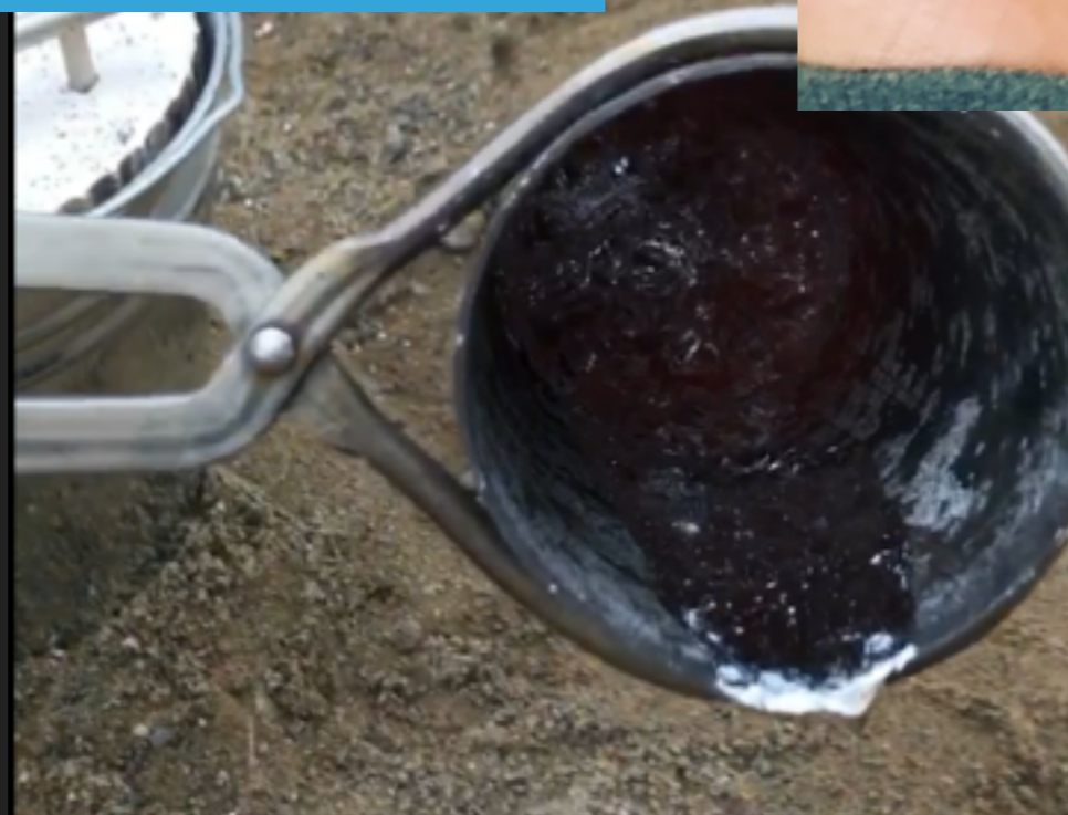
THEN THE MOST EXCITING PART OF THE MELTING CAME: POURING THE MOLTEN ALUMINUM INTO OUR STEEL CUPCAKE TRAY
