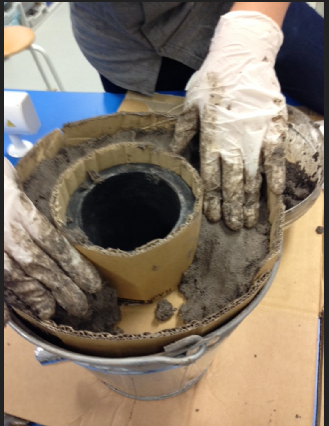
AFTER DRYING, WE THEN FINISHED OFF THE LID MADE OF CHAMOTTE
