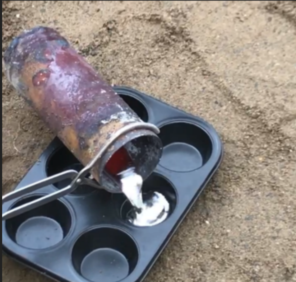
THEN THE MOST EXCITING PART OF THE MELTING CAME: POURING THE MOLTEN ALUMINUM INTO OUR STEEL CUPCAKE TRAY
